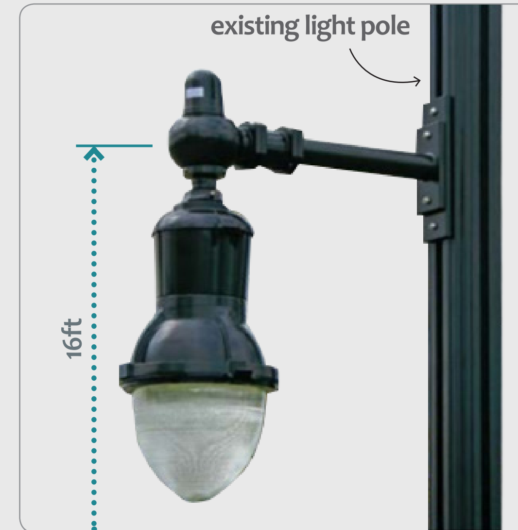
Arm + Fixture Attachment on (E) Light Poles ** 16ft above ground + Teardrop Fixture
