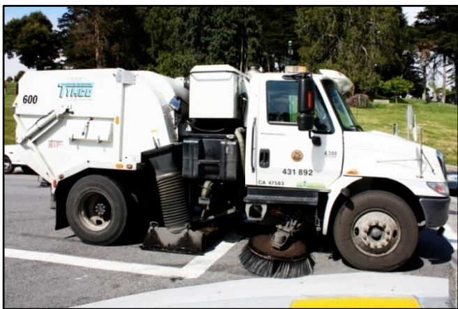
Mechanical Street Cleaning Sweeper
