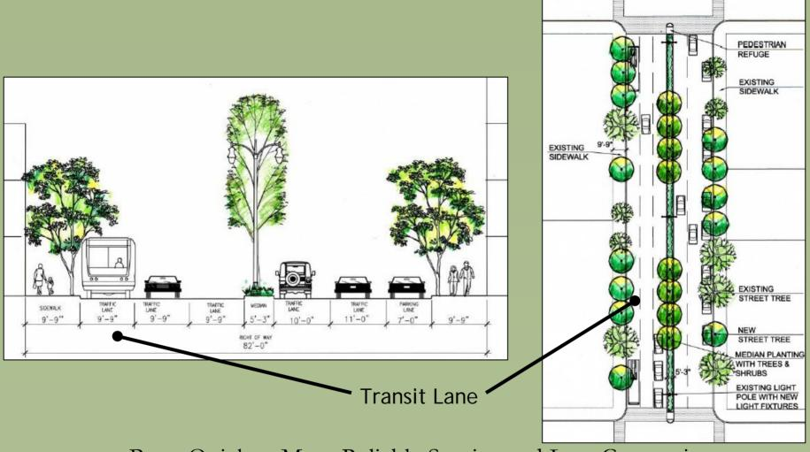
Pros: Quicker, More Reliable Service and Less Congestion Cons: Less Median Widening and One Less Bus Bulb Note: Wider Ped Refuges in Median Still Possible (4' to 5'-3'')
